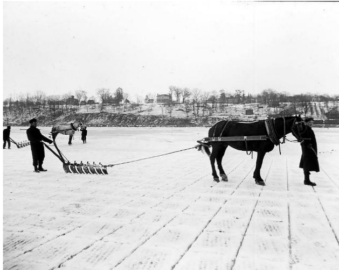
Horses pull the ice saws used to score ice with parallel cuts before final cuts were made with hand saws.
