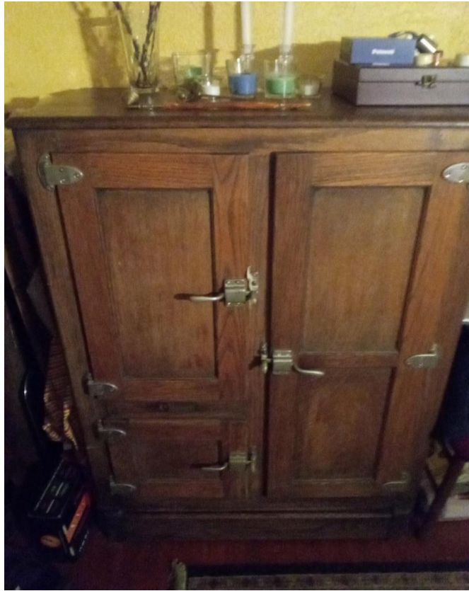
My relatively modern but less efficient, 1932 icebox. Note that the ice compartment is at the bottom. Bad idea.
